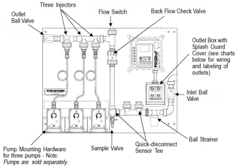
The charts below show standard receptacle wiring and labeling for conduit units based on model type:
