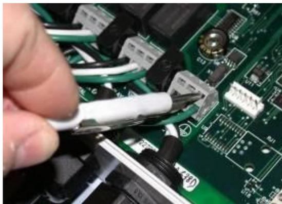
To operate the terminal blocks to remove or add wiring, insert a small screwdriver into the slot above each wiring connection and pry upward while removing or inserting the wire.
